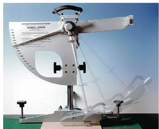
Figure 1 Wet pendulum test apparatus
